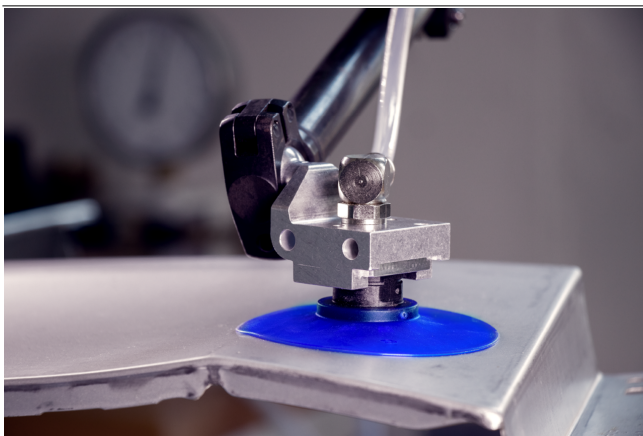
Holders for suction cup HT-SG in combination with bell-shaped suction cups SAX for handling sheet metal parts
